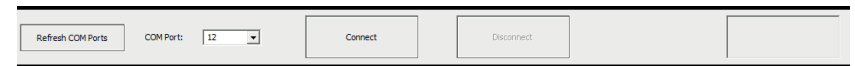
ECU connection area with algorithm ECU ready to be connected. COM port can be any number.
