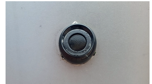
Flush mounting of a sensor/sleeve assembly to a vertical surface.
